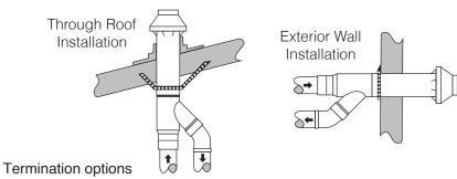
Concentric vent kits allows for both exhaust and intake pipes to penetrate the roof or side wall through only one hole.
